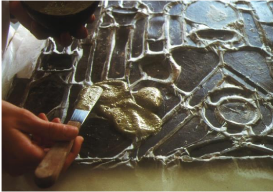
Fig. 2. Application of zeolite dressing with AB57 to remove the lime coating. Photo: Josep Gri.
